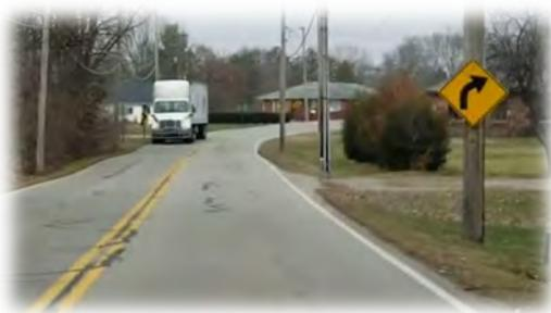
Curved sections within roadway corridor have limited shoulder widths and could use enhanced signing to warn motorists of the curves
